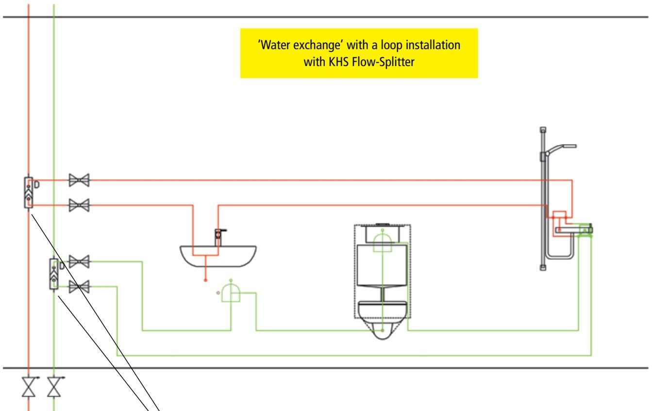
To exclude the problem of an ineffective and labour-intensive water exchange at the design stage, the installation shown above should be implemented in the bathroom area.
