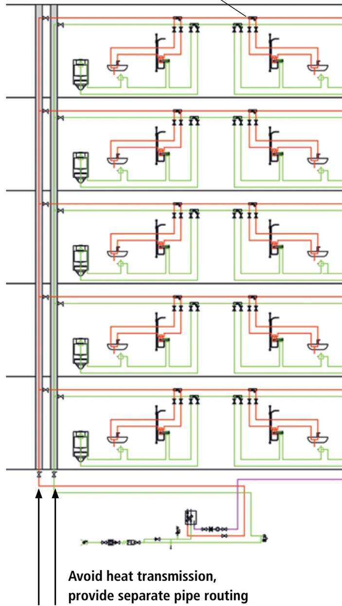
**Avoid heat transmission, provide separate pipe routing for PWC and PWH!**
