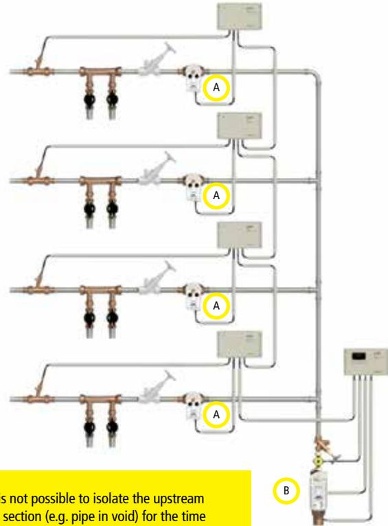
If it is not possible to isolate the upstream pipe section (e.g. pipe in void) for the time of maintenance on the valve, a maintenance shut-off (e.g. Figure 173) upstream of the valve is recommended.
