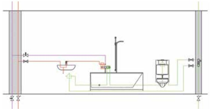
Heat transfer must be avoided at the design stage by laying hot pipes and cold-water pipes separately.
