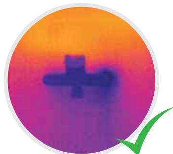
Mixing tap connected using a thermal separator.
