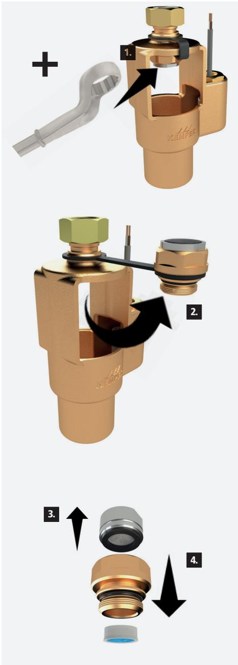
**1.** Use a size 27 ring spanner to unscrew the flow limiter.
