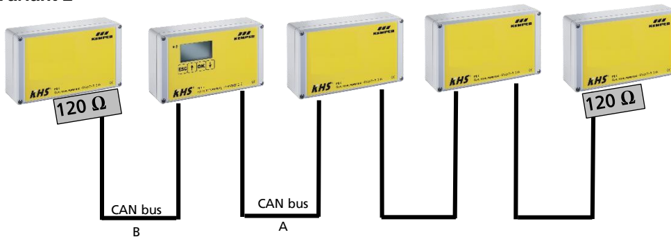
III. 5.3 Illustration of a CAN bus line with terminal resistor
